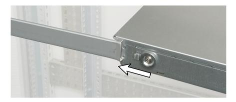
**9** Install a nut bar or mounting nuts on the front cabinet posts.
